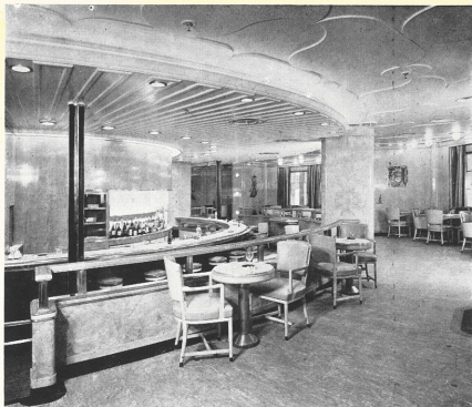
LEFT: First Class Cocktail Lounge in which nickel silver is used for the decorative balustrading, bar fittings, metal trim of bar and beading to columns. The hand-rail round the front is of cupro-nickel.
